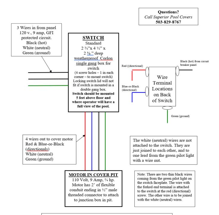
After final wiring, if the cover movement doesn't agree with the "Cover" – "Uncover" labels on the front of the switch, just reverse the positions of the red and blue-or-black directional wires on the switch.
