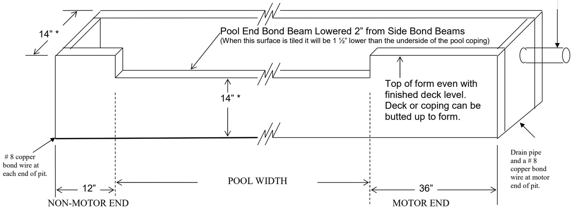
\* Note: A 14"x14" pit as shown is good for pool lengths up to 58 feet and widths up to 24 feet. Add 1" to these dimensions for every 8' interval of pool length over 56'. ( i.e. A 70' long pool would need a 16"x16" pit.) Add 3" to these dimensions for widths between 24 and 30 ft.
